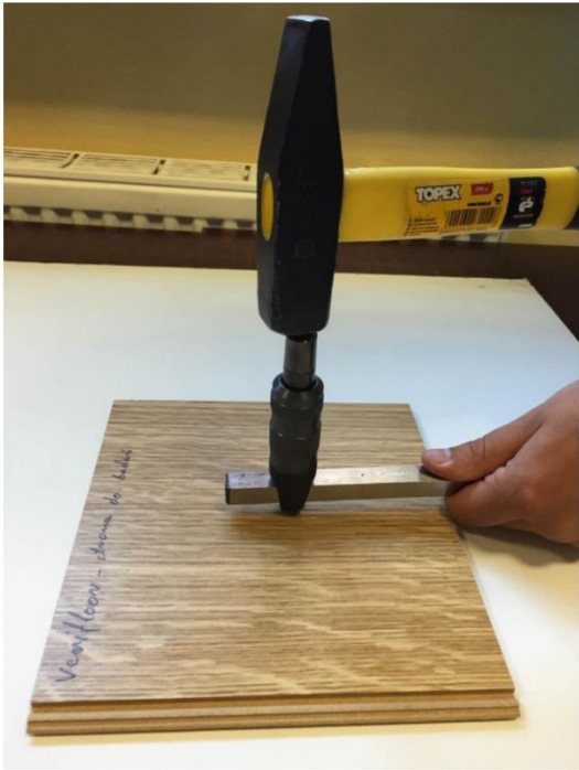
Fig. 2. Tools for Poldi hardness test: a) magnifier; b) Poldi hammer, C) reference sample, d) hammer
