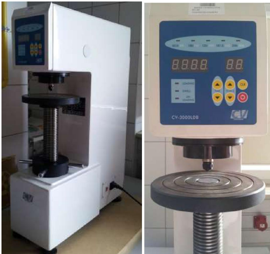
Fig. 1. Machine used for testing resistance to indentation with the Brinell method
